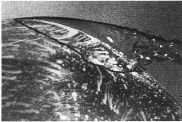
Fig. 4 Superposition photograph of the tip cavity and boundary layer characteristics
